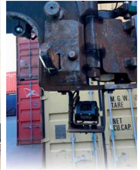
Twistlock camera for safe container handling.
