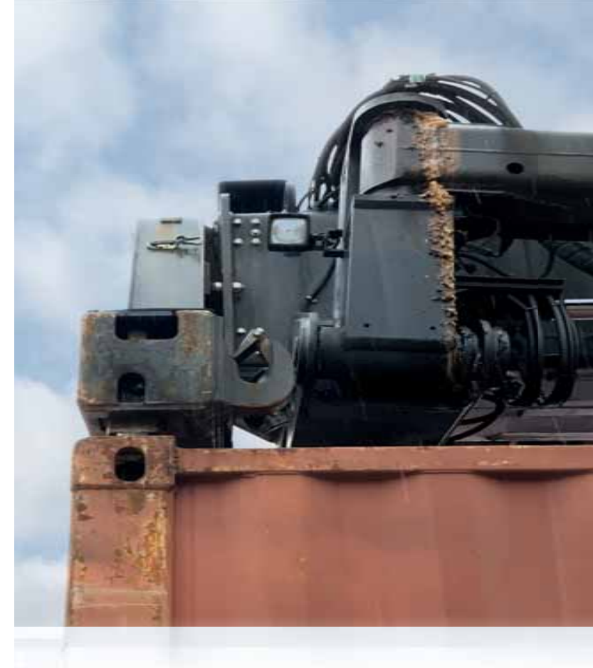
The cameras are mounted in such a way as to provide an optimum view onto the twistlocks.
