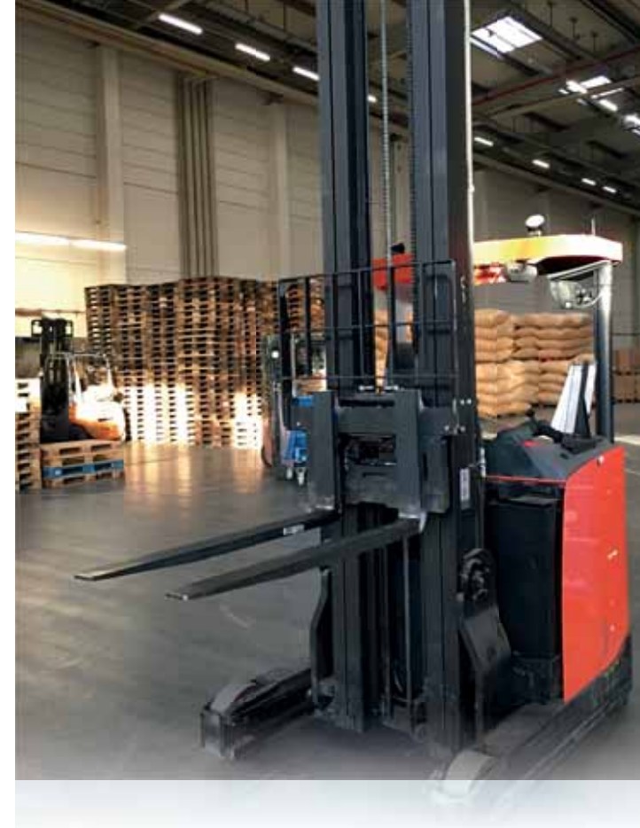
The fork camera on the reach truck allows the view onto both forks.
