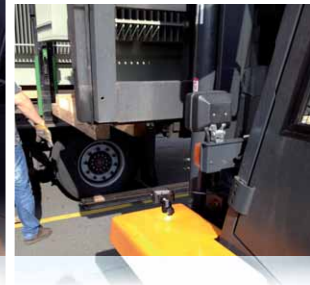
Camera-assisted truck loading.
