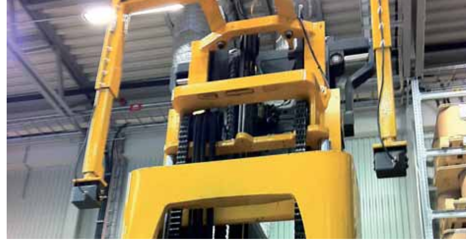
Cameras allow simultaneous viewing of the outer left- and right-hand side of the pallet.
