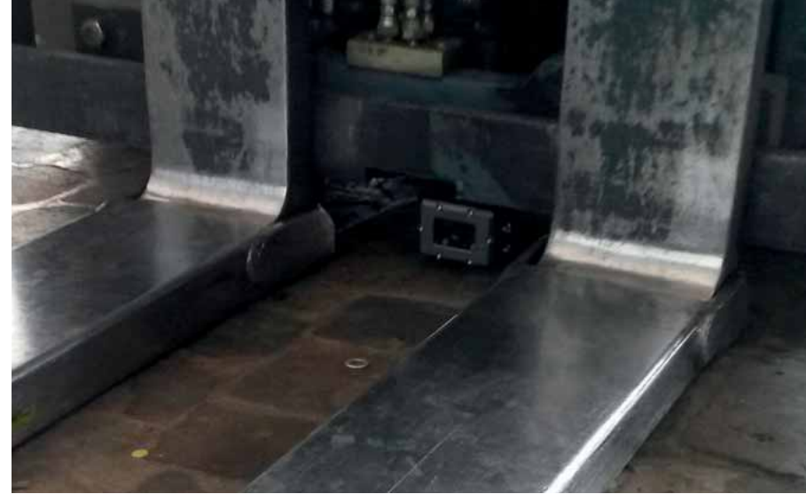
MVS system: MC3000B as optional fork carrier camera. Wide-angle camera MC7180N for lateral and rear view monitoring.
