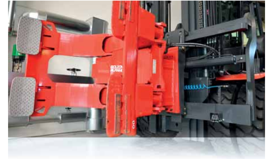
The camera allows visibility ahead of or below the load.
